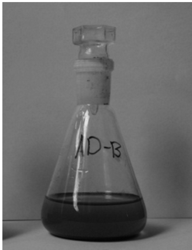
Fig. 1. Sol–gel distribution of ASUD-99 detonation nano-diamonds in toluene.
